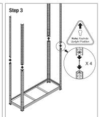
Place MDF board on bottom shelf to minimise buckling. Join the upper legs to the lower legs with the connector pins. Note: The legs are designed to sit directly on top of each other – don't overlap them. Handy Hint: Flathead screwdriver may be used to tap in connector pins.
