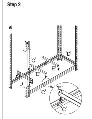
Use shelf bracket 'B' for the side brackets using the shelf bracket from Step 1 as a guide for height. Allow 1 keyhole free from the ground as shown in the diagram. Use same shelving brackets for opposing sides as shown in the diagram. Place braces 'E' as shown.
