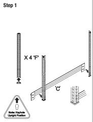
Place foot end caps onto the bottom of the legs 'F'. Note upright position. Place shelving bracket 'A' onto the legs 'F'. A rubber mallet can be used to lightly tap all brackets into the keyholes of the legs into place. Allow one keyhole free between the foot cap and the shelving bracket.
