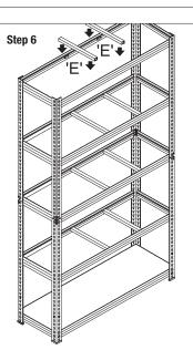
Apply remaining brackets as above to desired height. Ensure that the braces 'E' are fixed to all shelves.
