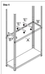
Fix brackets 'D' so that the top rivet sits on the upper legs and the bottom rivets sit on the lower legs. Repeat with brackets 'C', followed by braces 'E' as shown.
