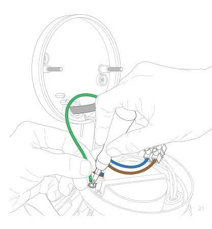
For safety and the proper operation of your Ring Floodlight Cam, the fixture must be properly earthed.
