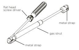
**note:** the gas strut can be adjusted by moving the bracket on the door forwards or backwards.
