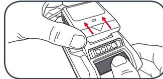
5 When removing the charger from the battery, first press the battery release tab, then slide the charger from its position.
