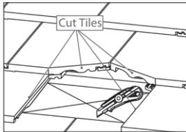
Remove single tile and cut other tiles as required. If the roof is sarked, cut and fold sarking to provide a 300mm opening.
