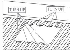
Cut a 300mm square or round opening around centre of position marks. Turn up corrugations or pans on low and high sides to prevent water ingress.
