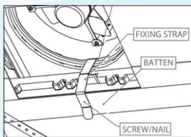
Use the fixing strap to secure the ventilator to the bottom batten.
