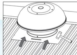
Slip ventilator under ridge capping and form flashing into roof corrugations. In BAL zones ensure there are no gaps greater than 3mm.
