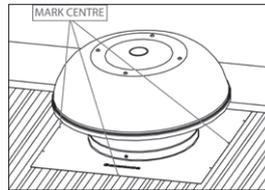
Select suitable position, slip the top edge of flashing under ridge cap and mark position. Back flashing must be used if positioned lower down on the roof.
