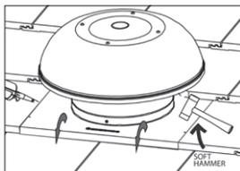
Slide under tiles above ventilator. Fold and form flashing to tiles below. Ensure no gaps greater than 3mm are present. Silicone beading can be applied for weatherproofing in non-BAL areas. **THIS CANNOT BE DONE IN BAL ZONES DUE TO COMBUSTIBLE NATURE OF SEALANTS.**
