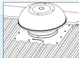
Use silicone sealant in non-BAL zones. **NOT TO BE DONE IN BAL ZONES DUE TO COMBUSTIBLE NATURE OF SEALANTS.** Secure flashing with TEK screws or rivets along three exposed edges.
