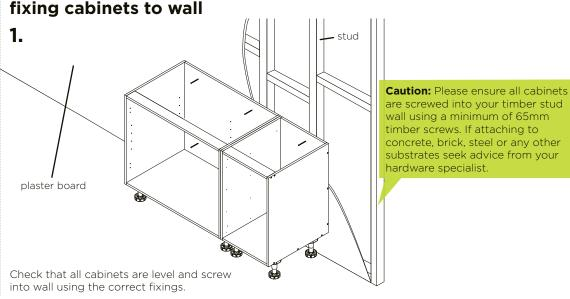
are screwed into your timber stud wall using a minimum of 65mm timber screws. If attaching to concrete, brick, steel or any other substrates seek advice from your hardware specialist.
