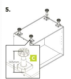
Set height of the adjustable feet to 145mm.
