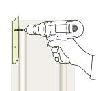
If installing a handle on a wall cabinet door, line up the bottom of the template with the bottom of the door and use the bottom hole as your first marking point.
