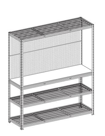
Step 7: Lay the wire shelf between brackets as shown.
