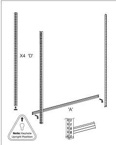
Step 1: Add Foot End Caps to bottom of Legs 'D'. Slot Brackets 'A' into the bottom of Legs 'D' as shown in the diagram. NOTE: Flat edges face outwards. Lock rivets to the bottom of the keyhole by tapping the Brackets with a rubber mallet.
