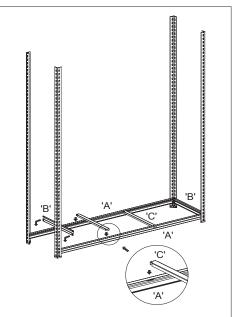
**Step 2:** Slot Brackets 'B' into the bottom of Legs 'D' as shown in the diagram. Slot Braces 'C' into position through the holes provided on Brackets 'A'. NOTE: Flat edges face outwards. Lock rivets to the bottom of the keyhole by tapping the Brackets with a rubber mallet.
