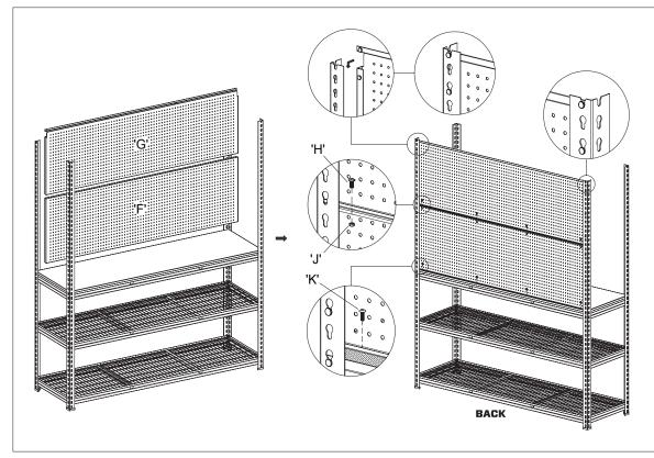
Step 5: Slot Bottom Pegboard 'F' and Top Pegboard 'G' into the keyholes above the benchtop as shown in the diagram. Secure the two pices of pegboard together in the middle with the provided bolts 'H' and nuts 'J' and then fasten the bottom pegobard to the timber benchtop using the M5 x 16mm Self Tapping Screws 'K' provided. Please note when fixing the bottom pegboard to the timber benchtop it is recommended that you drill a pilot hole using a 3mm drill bit.
