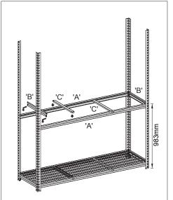
**Step 3:** Assemble the benchtop frame by slotting brackets A and B followed by braces 'C'. **Please note:** All brackets for this step need to be slotted into the 25th and 26th keyhole from the bottom of part 'D' (legs).
