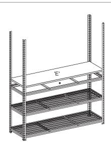
**Step 4:** Repeat Steps 1 and 2 for the middle shelf. Lay the wire shelf and Timber Benchtop 'E' between brackets as shown in the diagram.
