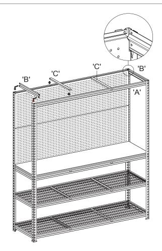
**Step 6:** Slot in Bracket 'A' and Brackets 'B' into the top of Legs 'D' as shown in the diagram. Slot Braces 'C' into position through the holes provided. NOTE: Flat edges face outwards. Lock rivets to the bottom of the keyhole by tapping the Brackets with a rubber mallet.
