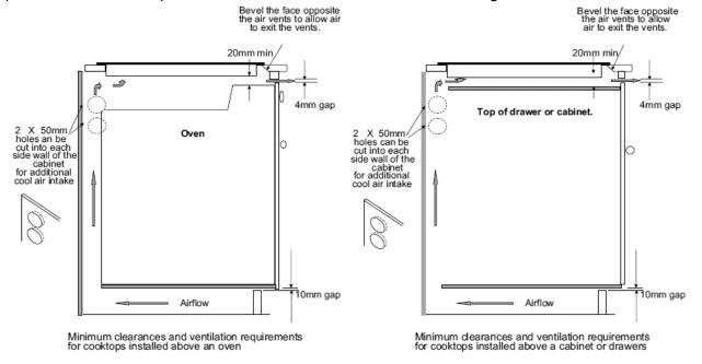
A board must be placed a minimum of 20mm below the cooktop that prevents anyone from touching the underside of the cooktop. Take care that there is adequate ventilation for air exchange to the inductive elements (at least 20mm).
