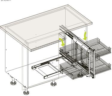
Remove the screws from the handles, position the handles on the frame as pictured above and fix into place. Place the top rail of each wire basket onto the small hooks on the frame to complete installation.
