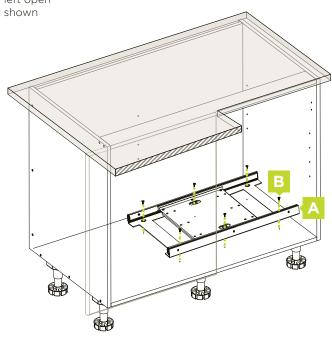
Align the sliding track frame (A) with the pre-drilled holes and using the 6mm wood screws (B), fix the sliding track to the bottom of the cabinet.
