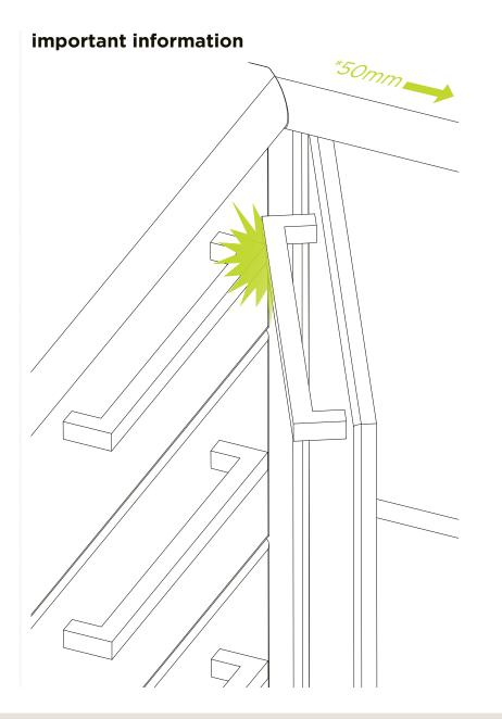
**NOTE:** Some handles in certain configurations can collide with each other when doors are open, potentially causing the blind corner cabinet doors to not open wide enough to access the pantry.
