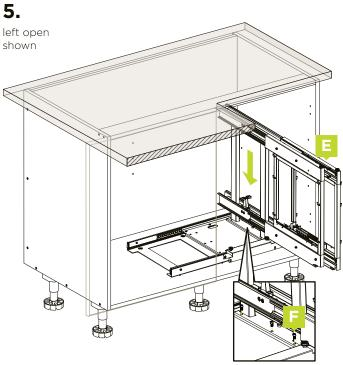
Move the sliding track frame closer to the cabinet side panel. Screw the basket frame (E) securely onto the sliding track frame using the hex screws (F) and allen key provided.
