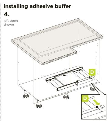
Stick the adhesive buffer (D) onto the back of the front support rail just below the top cut out, as pictured above. This will absorb the impact of the rear roller when opening.
