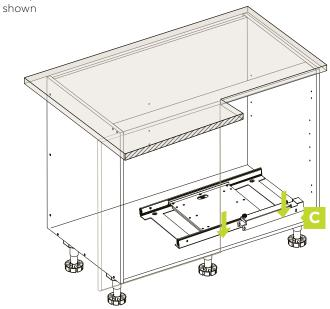
Loosen the 2 screws on the front of the sliding track frame so they are sitting 3mm out. Slide the holes in the front support rail (C) over the screws, ensuring the top cut out is closest to the cabinet side panel, as pictured above. Secure into place by tightening the screws.
