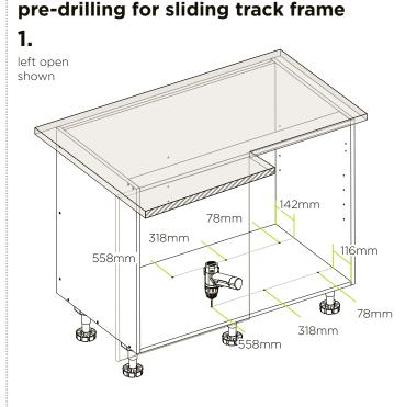
Mark out and pre-drill six holes on the bottom cabinet panel as per the diagram above. Use a 2mm drill bit to pre-drill holes to a depth of roughly 2.5mm.
