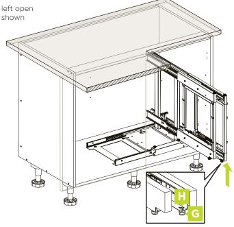
Attach the front roller wheels (G) to the bottom of the basket frame using the hex nuts (H) provided. Use the front round hole for the roller on the right side of the frame. Use the elongated hole for the roller on the left side of the frame.
