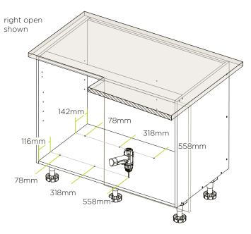
The measurements are mirrored for right hand open, as pictured above.
