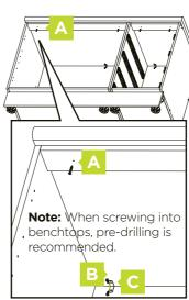
Fix the benchtop to the back of the cabinet using 90° angle bracket and 14mm screws. Fix the support rail using 28mm screws through into the benchtop
