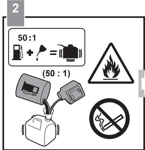
Pre-mix 2-stroke engine lubricant and unleaded petrol in a clean container approved for petrol at a 50:1 ratio.
