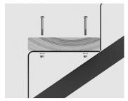
Install each timber tread using M8 x 60 mm cup head bolts, nuts and washers.
