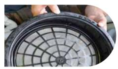
**ACTION**: Remove the filter and hose clean. The use of a scrubbing brush may be required to remove dry and stubborn debris.
