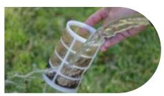
ACTION: Turn off the power point, remove primary filter cap, remove and clean filter replace ensuring the cap is tightened.
