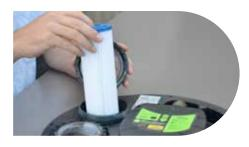
ACTION: To check if you have a cartridge filter installed or to replace. Turn off the power point, remove secondary cap, remove and clean or replace with new filter, ensure the cap is tightened.
