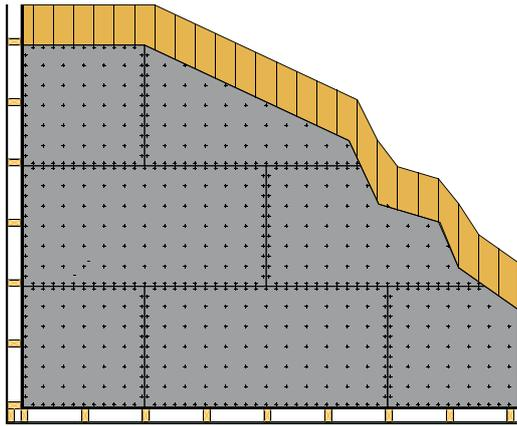
Note: Underlay sheets to run perpendicular to floorboards. Stagger joints in underlay sheets
