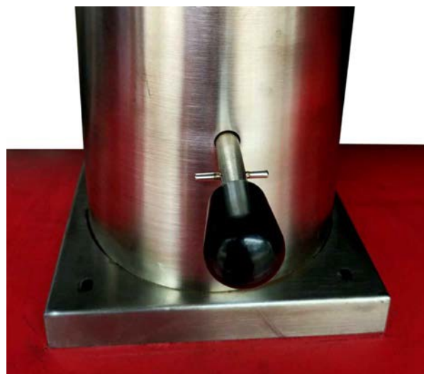
Damper in fully closed position
