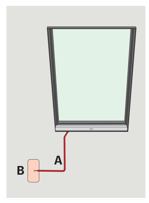
A junction box or an outlet box (not provided with skylight) is required for permanent connection of the 20 ft (6 m) skylight power cable.
