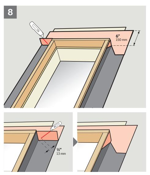
Wrap the curb at top frame of skylight with VELUX roofing underlayment ZOZ 216 and create proper water-shedding lap.
