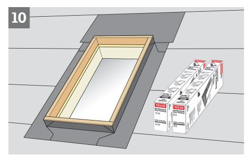
For thin roofing materials, use flashing ECL. ECL is designed for roof pitches 10° - 60° (2:12 - 21:12). For profiled roofing materials, use flashing ECW. ECW is designed for roof pitches 14° - 60° (3:12 - 21:12).
