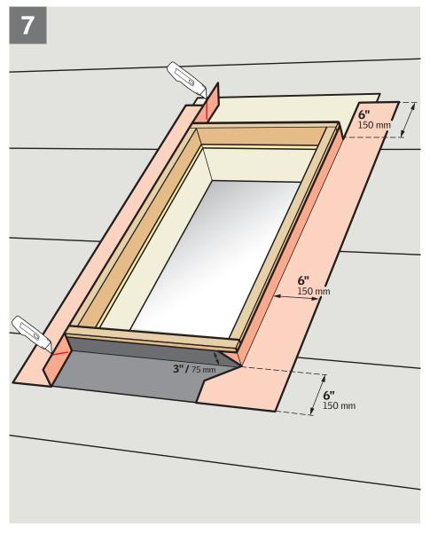
Wrap the curb with VELUX roofing underlayment ZOZ 216 and create watershedding laps over felt at bottom and sides of skylight 6, 7.
