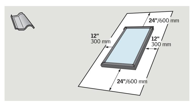
Maintain illustrated clearances between skylight frame and critical areas such as valleys, ridges, slope changes and roof-to-wall-intersections.
