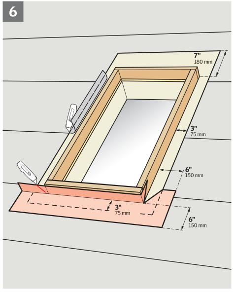
Skylight curbs should be completely wrapped in self-adhesive membrane to ensure waterproofing. To achieve this waterproofing, use VELUX roofing underlayment ZOZ 216 (9" wide). ZOZ 216 must be applied before installing the flashing.
