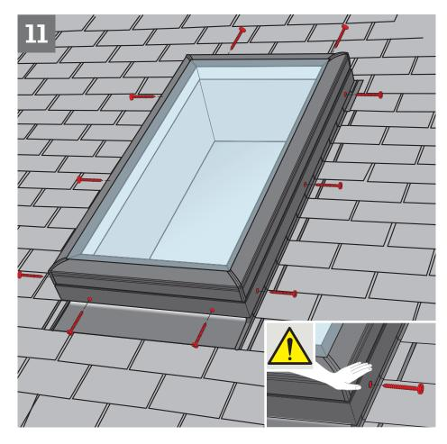
Center the skylight on top of the curb and secure with #8  $1\frac{3}{4}$ " (45 mm) pan head stainless steel screws provided. Screws will penetrate the curb by at least  $\frac{3}{4}$ " (19 mm).
