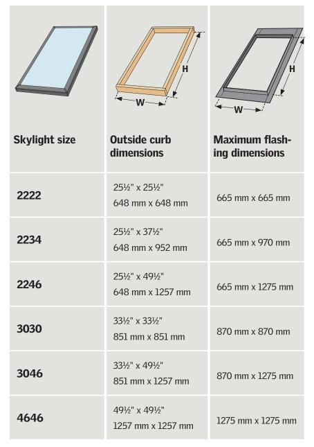
Build curb according to measurements in the chart. Use lumber with an actual thickness of  $1\frac{1}{2}$ " (38 mm) and a minimum height of  $3\frac{1}{2}$ " (90 mm). Curb height and attachment should comply with building codes and regulations and be secure enough to transfer the skylight loads to the framing members.
