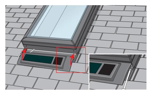
Install solar panel as shown and secure the screws.
