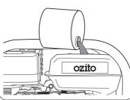
3. Unscrew the dipstick and fill the oil tank until it reaches the max indicator on the dipstick. Oil tank capacity is 0.60L. Ensure the dipstick is screwed back on once filled.
