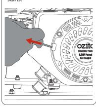
8. Once started move the choke to the right (open position) and the throttle lever to the right (slow position) and idle for 3min.
