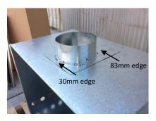
Step 6: Screw outer top panel into place.1 x large return facing upwards at the front,3 x small returns facing downwards.
