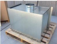
**Step 2:** Screw inner left, inner right and inner back panels together, returns facing outwards.
