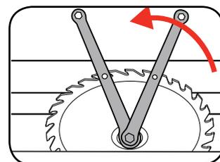
**IMPORTANT!** TURN THE BLADE BOLT IN THE DIRECTION OF ROTATION OF THE SAW BLADE.
