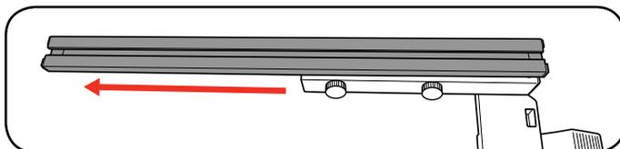
**Note:** Rule of thumb: The rear end of the stop comes up against an imaginary line that begins roughly at the centre of the blade and runs at an angle of 45° to the rear.
