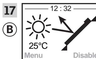
The display shows the program mode including current temperature and time.
