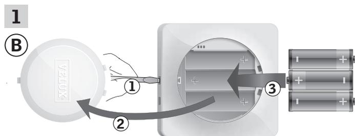
Remove the battery compartment lid by pressing the release button with a screwdriver as illustrated ①, ②.
