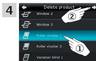
4 Tap the product to be deleted, in this case "Roller shutter 1" ①. **Note:** The individual products can be identified by tapping the icon. See also the section *Finding products*. Tap ⇒ ②.
