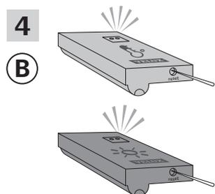
**4** Prepare sensors for registration: Press the button at the bottom of the sensor with a pointed object for at least 5 seconds until the diode flashes.
