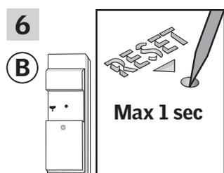
Press briefly the RESET button on the back with a pointed object to register the new product.
