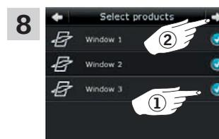
8 Scroll down the display and tick the windows to be included in the program ①. **Note:** The individual products can be identified by tapping the icon. See also the section *Finding products*. Tap ⇒ ②.
