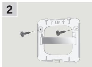
Fit the back section onto the wall with the two screws supplied.
