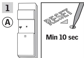
Press the RESET button on the back with a pointed object for at least 10 seconds to prepare the products for copying.
