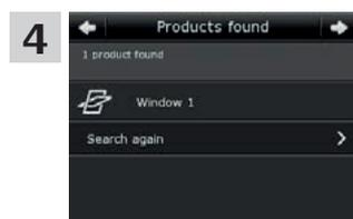
Tap ⇒ when the control pad has found **all** products. **Note:** Tap "Search again" if the control pad did **not** find **all** products and follow the instructions in the display. Go to the section *If the initial set-up fails* if the control pad still cannot find all products even if they are connected to power.
