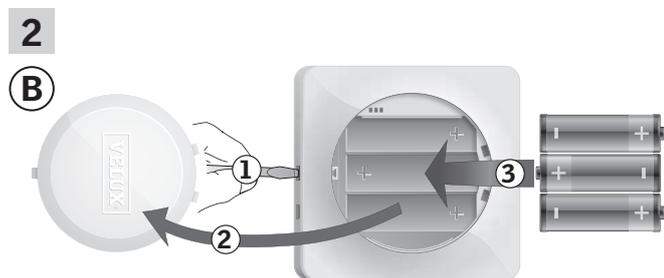
Remove the battery compartment lid by pressing the release button with a screwdriver as illustrated ①, ②. Insert batteries (type AA/LR6) ③. Replace lid.
