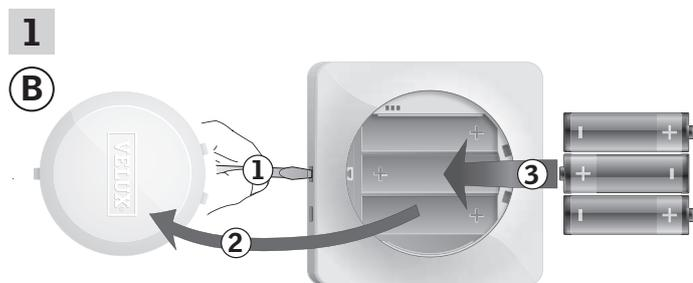
Remove the battery compartment lid by pressing the release button with a screwdriver as illustrated ①, ②.
