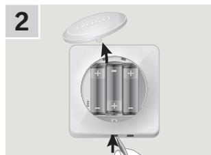
Remove the battery compartment lid by pressing the release button with a screwdriver as illustrated.
