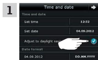
Time switches automatically from summer time/daylight saving time to standard time and vice versa. This function can be disabled by removing the tick for "Adjust to summer time".
