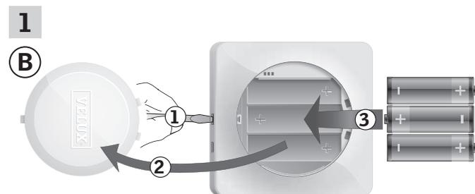
Remove the battery compartment lid by pressing the release button with a screwdriver as illustrated (1), (2).
