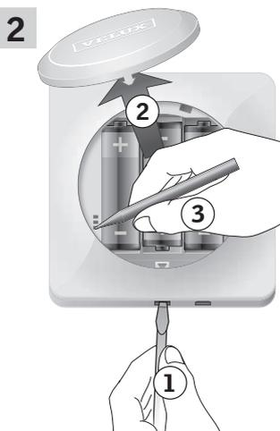
2 Remove the battery compartment lid by pressing the release button with a screwdriver as illustrated ①, ②. Press the RESET button on the back of the control pad with a pointed object for at least 5 seconds ③. Replace lid.
