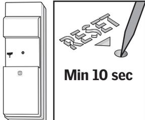
Press the RESET button on the back with a pointed object for at least 10 seconds to prepare the products for registration.
