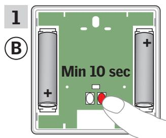
Press the RESET button on the back for at least 10 seconds to prepare the products for registration.
