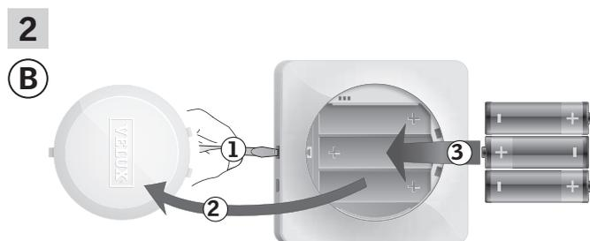
Remove the battery compartment lid by pressing the release button with a screwdriver as illustrated ①, ②. Insert batteries (type AA/LR6) ③. Replace lid.
