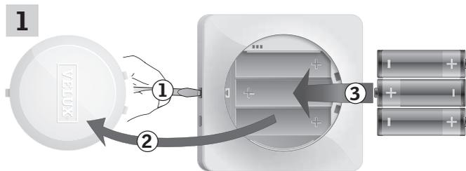
Remove the battery compartment lid by pressing the release button with a screwdriver as illustrated ①, ②. Insert batteries (type AA/LR6) ③. Replace lid.
