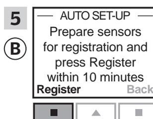
**5** Register sensors in the controller: Press "Register" to register the two sensors.
