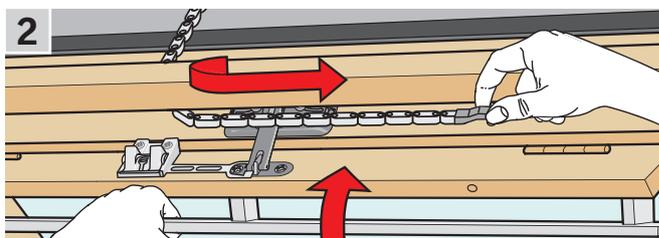
When the power has been reconnected or the battery has been recharged, you must re-engage the chain.
