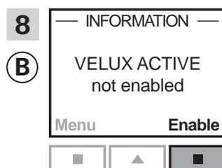
**8** The display shows that the program VELUX ACTIVE has not been enabled. Press "Enable" to start registration of sunscreening products in the controller.
