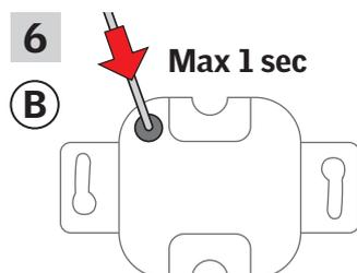
Press briefly the SET button on the back with a pointed object to register the new product.
