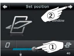
Drag the slider or tap the bar to open window to desired position. The position from 0-100 is shown in the bottom right corner ①.
