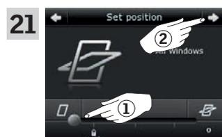
21 Drag the slider or tap the bar to set the opening of the windows to 0%. The position from 0-100 is shown in the bottom right corner ①.
