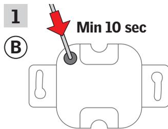
Press the SET button on the back with a pointed object for at least 10 seconds to prepare the products for registration.
