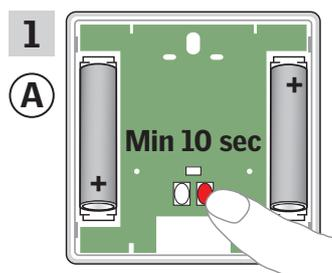
Press the RESET button on the back for at least 10 seconds to prepare the products for copying.
