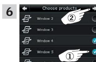
Scroll down the display and tick the windows in the room ①. **Note:** The individual products can be identified by tapping the icon. See also the section *Finding products*. Tap ⇒ ②.
