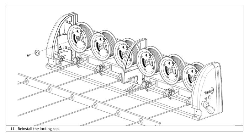
12. Unwind line from the new Spool Assembly and thread it around the Roller and through the locking Bar. Use the other spools as a reference.
