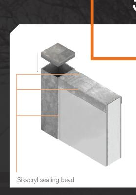
// Prepare the surface of the panels to ensure they are clean and ready to paint. Lightly scuff the metal posts with a scouring pad and ensure they are clean. Use Sikacryl Super (or equivalent) gap sealant between the joins of the Fence Panels to minimize the joint before painting.
