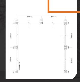
// Make up each of your posts according to step 1 using the 89mm x 89mm square posts and the Panel Channel. Each post is made according to its position in the layout and is either a 180 degree, 90 degree or an end-of-line combination.
