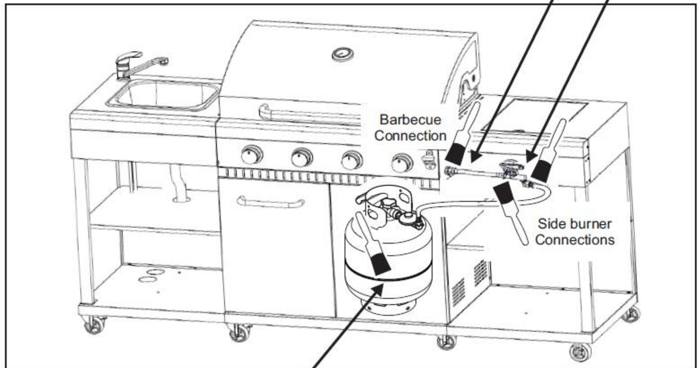
If there is a leak anywhere on the gas cylinder, do not use the cylinder. Locate the leaking cylinder outdoors away from sources of ignition, then contact your local gas authority or cylinder exchange provider to arrange disposal.
