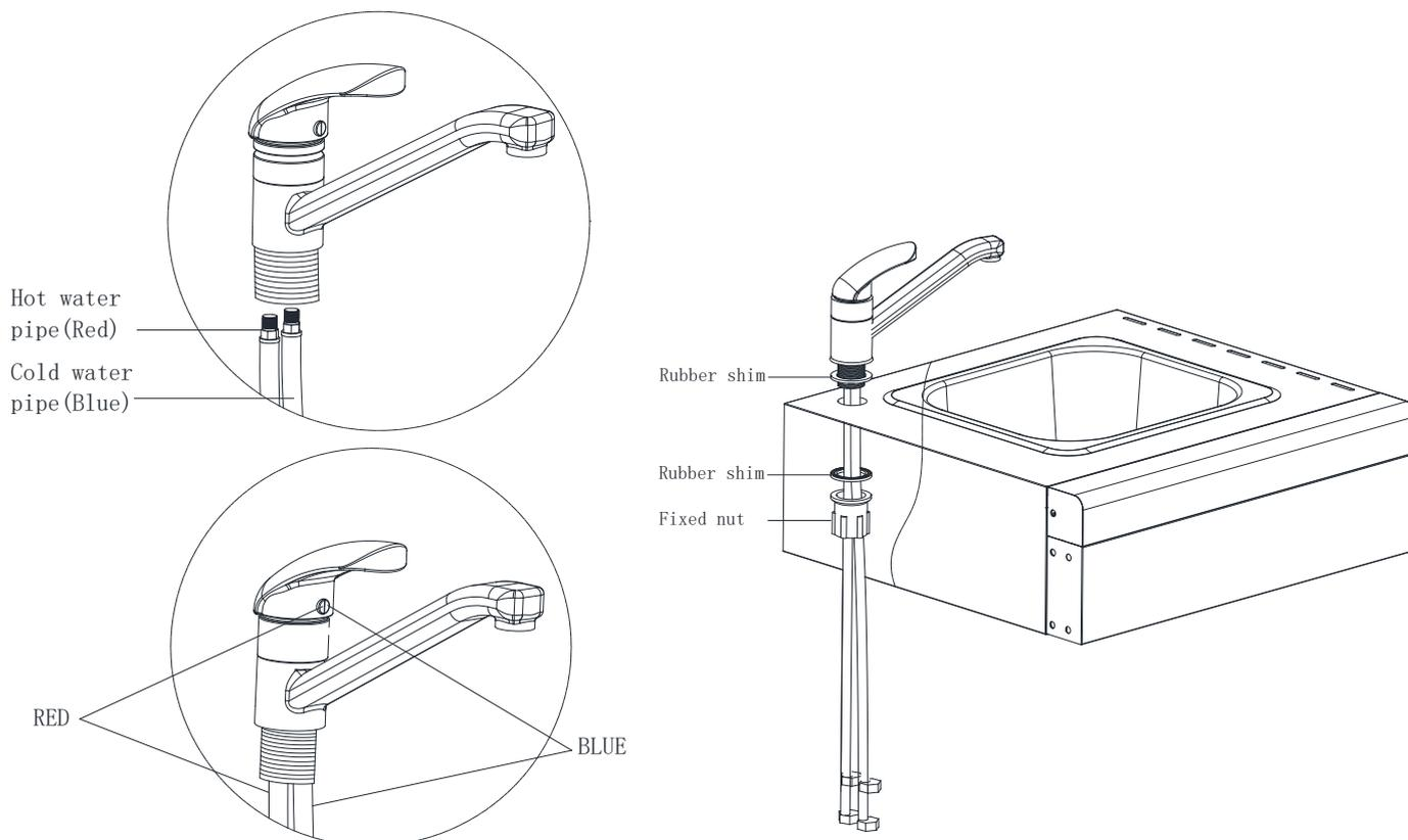
Assemble the water pipe: the left is red and the right is blue.
