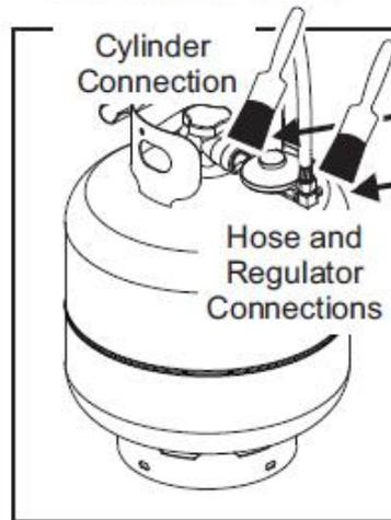
Soap bubbles will appear if there is a gas leak. In case of a leak, turn off the gas supply. Tighten any leaking fittings, then turn the gas supply on and re-check.
