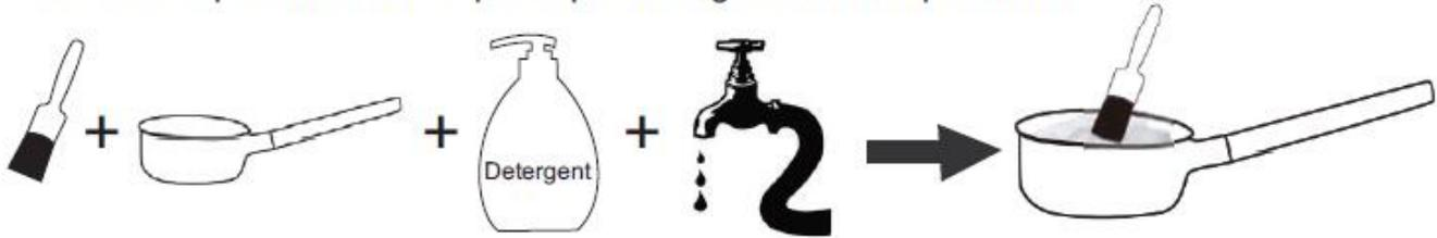
Make sure the control knob on the barbecue is off and the gas valve on the cylinder is off before mixing the soapy solution.
