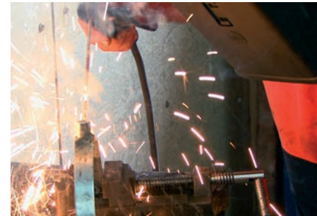
Welded Nut Clip – Welding undermines the strength of the steel and is prone to corrosion.
