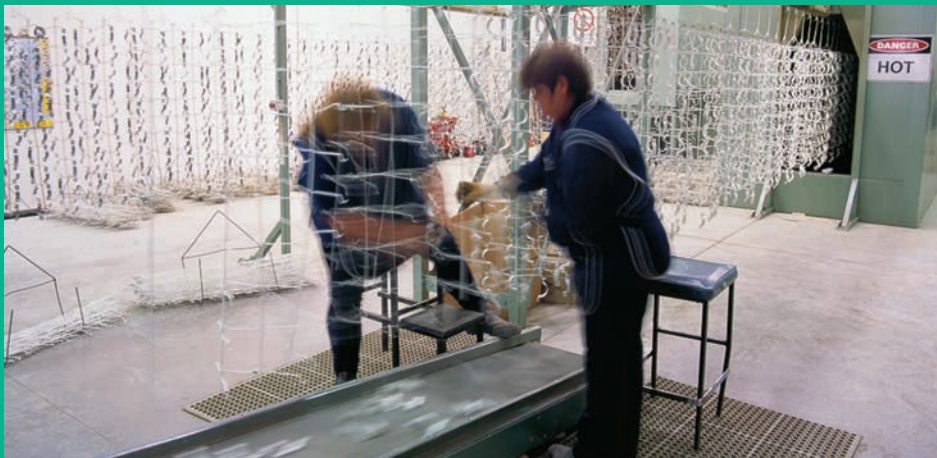
Abey's manufacturing facility showing the powder coating operation.
