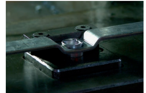
Machine Pressed – Machine pressed clipping products provide a greater strength than welding and are less prone to corrosion.
