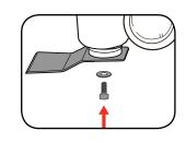
3. Tighten locking bolt with hex key.
