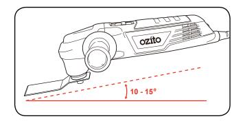
Allow the scraper to do the work; do not apply heavy pressure to the multi function tool. This may cause the multi function tool to overload or cut into the surface of the workpiece.
