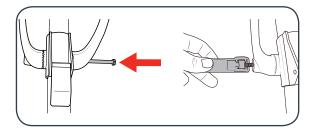
3. Select the most comfortable position and close the lever to lock the auxiliary handle in position.
