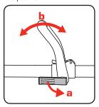
2. (a) Open the mounting bracket lever and (b) slide the additional handle into the required position, close to lock into position.
