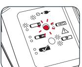
5. The charger LED will illuminate green once the battery is fully charged.
