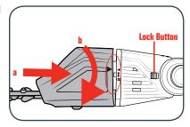
**Note:** The Lock Button will "CLICK" back to the left (original position) when the trimmer head is correctly secured in place.
