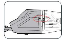
(a) Press the trimmer head against the motor head. This will cause the lock button to be pushed to the right.
