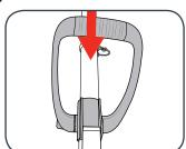
Pass the bolt through the auxiliary handle and screw the lever to the end of the bolt.
