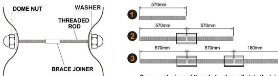
Screw each piece of threaded rod equally into the joiner until tight
