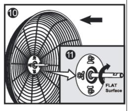
12 Slide and push the fan blade onto the spindle. Push it until the end of the fan blade hole is aligned with the end of the spindle.
