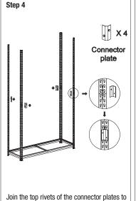
the bottom keyholes of the upper legs and bottom rivets of the connector plates to the top keyholes of the lower legs. Gently tap the connector plates in place with a mallet and a screw driver on the notch.
