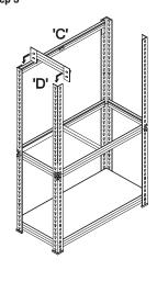
Fix brackets 'C' at the very top allowing room for the MDF board to sit flush against the legs. Repeat with brackets 'D'.
