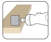
WARNING: PLACING EXCESSIVE LOAD ON THE ROTARY TOOL WHILE IT IS RUNNING AT LOW SPEEDS MAY CAUSE IT TO OVERHEAT AND THE MOTOR TO FAIL.
