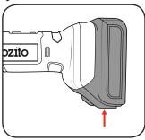
2 To remove the battery, press the battery release button and then remove the battery.
