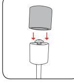
2 Slide the sanding drum onto
