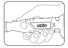
5 Gently apply the tip of the accessory to the work piece.
