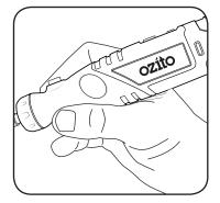
4 For heavy work like cutting or grinding, hold the rotary tool in the palm of your hand.
