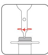
Note: Do not over-tighten the screw as it could result in damage to the cutting disc.
