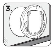
Install exterior frame into hole and slide interior frame over top to required fit.
