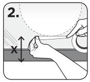
Mark height (x) on door / panel with tape or similar. Cut required hole out above. Hole sizes below: 1158 Small: 250mm (9.8") 1159 Medium: 388mm (15.2")
