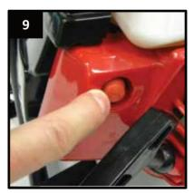
When ready to stop the pump, move the throttle back and press the "STOP" button until the engine stops. If not using the engine again for a while turn the fuel tap to the closed position.
