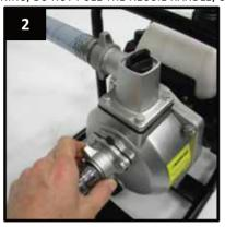
Using the connectors provided, connect the inlet and outlet hoses to the pump (hose not included).
