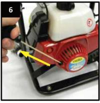
Pull the recoil starter in the direction shown until you feel resistance. Now pull the recoil starter hard several times until the engine fires briefly.
