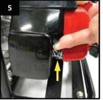
Lift the choke lever to the "CLOSED" up position.
