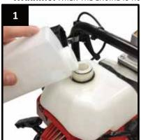
Only use 40:1 fuel to oil mix ratio. Mix the fuel and oil in the bottle provided, Unscrew fuel cap and fill the fuel tank with the mix. Replace the fuel cap. Wipe clean any spillages.
