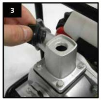
If the supply hose does not fill the pump chamber, the pump will need to be primed by filling with water manually. Unscrew the priming cap and fill with water. Screw the priming cap back on tightly.
