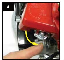
Turn the fuel supply tap to the "OPEN" position.
