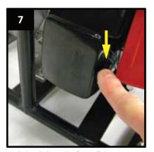
Push the choke to the "OPEN" down position and pull the recoil until the engine starts.
