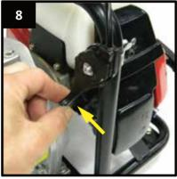
Let the engine warm up. When ready to start pumping, push the throttle forward to the "H" position.
