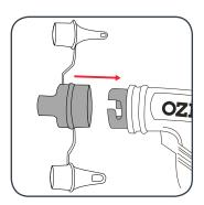
3 Connect inflation adaptor to workshop blower housing and rotate adaptor clockwise until it clicks into locked position.
