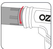
5 To remove blower nozzle, rotate in anticlockwise direction.
