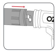
4 To lock into place, rotate nozzle in clockwise direction until nozzle clicks into place.
