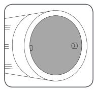
3 Line up the internal nozzle nodes with workshop blower housing and slide into place.
