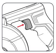
2 To stop the blower release the on/off switch.
