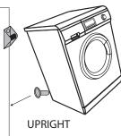
You will need to pack at the bottom spacers by the same thickness as the batten to keep the dryer upright and level.
