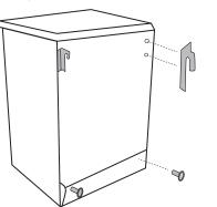
When locating the mounting brackets onto the dryer back panel, you may notice only one screw hole. If this is the case, you will need to take the other self-tapping screws to push and pierce the dryer back panel. (this will locate the hole beneath the back panel). Continue to turn the self-tapping screws until tightens. Once done, in the same manner fit the spacers to the back of the dryer.
