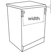
Note the measurements from the top of the dryer to the top of the dryer bracket and the distance between the dryer brackets etc.
