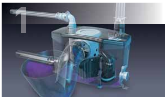
1 When the toilet is flushed the water level rises and the Saniflo pump operates automatically.
