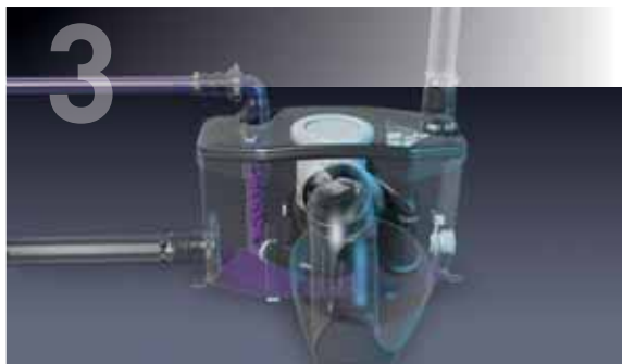
3 The resultant slurry is pumped out via the impeller on the bottom of the motor, through a pipe of just 20-25 mm in diameter, then stops automatically.
