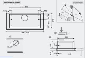
Method of Installation: Built into overhead cupboards
