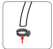
2. Securely attach the lay flat hose to the pumps universal adaptor (not supplied), and tighten.
