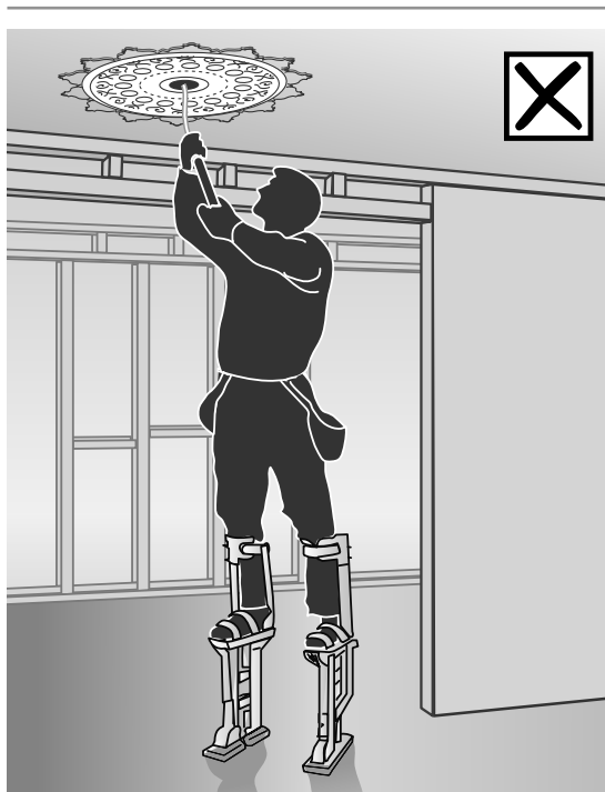
Figure 26 (a) Hazard: plasterers' stilts
