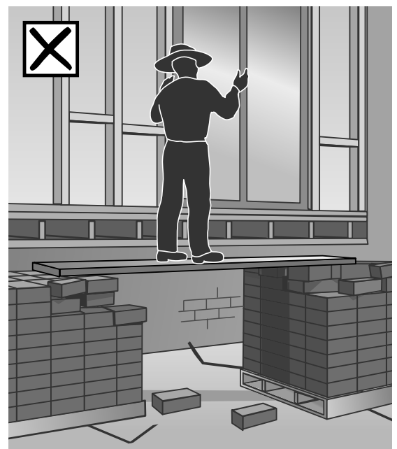
Figure 28 Hazard: makeshift means of gaining height. A safer alternative: trestles as shown in Figure 26 (b)
