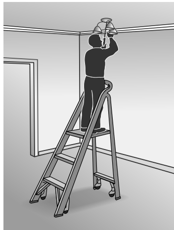
Figure 27 (b) A safer alternative: select the right ladder or step platform for the job
