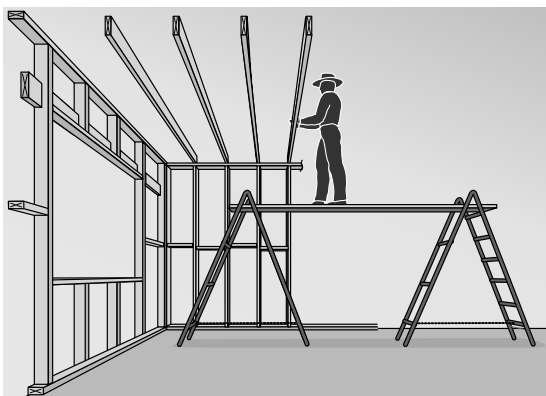
Figure 13 Installing ceiling or upper level floor joists
