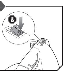
To stop the engine, toggle the switch to the "STOP"
