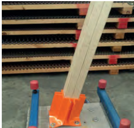
Safety base tested to 3160 Newtons without failure
