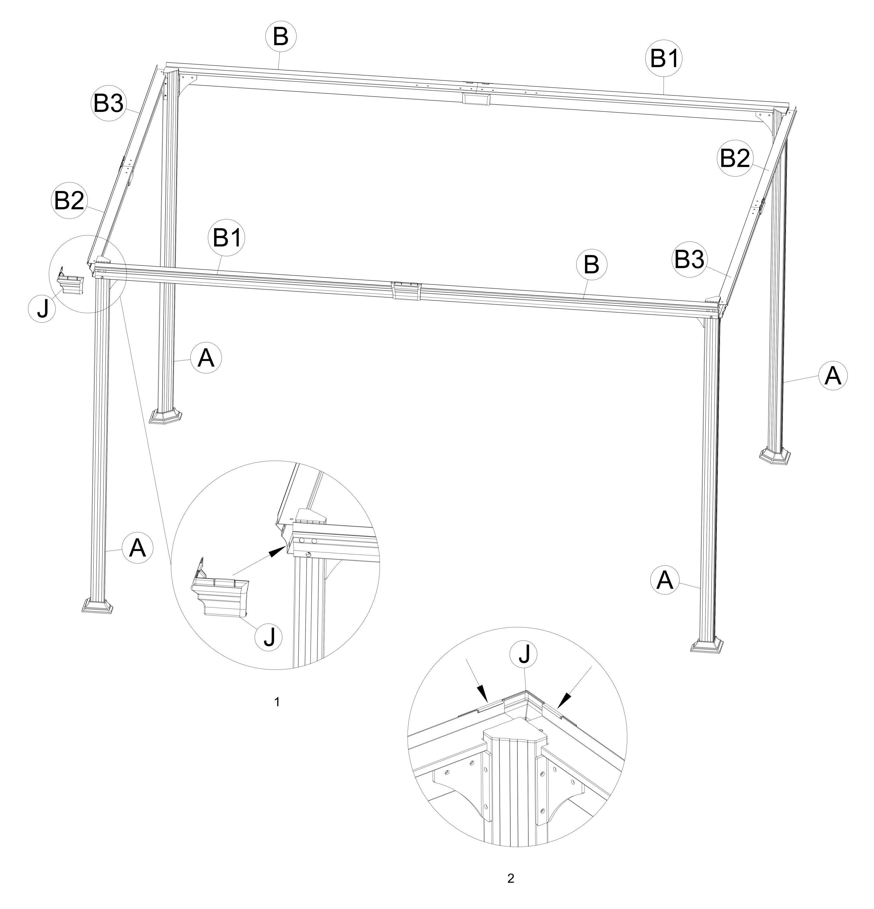
Secure the four package plate(J) with the ring beam (B1) and ring beam (B2), push.
