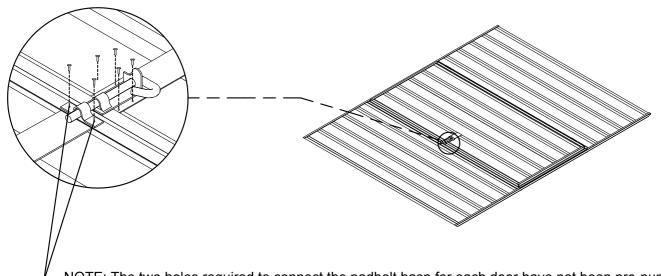
NOTE: The two holes required to connect the padbolt hasp for each door have not been pre-punched, to allow for proper alignment. position each hasp centrally over the padbolt shaft, and drill 3mm holes and secure with screws
