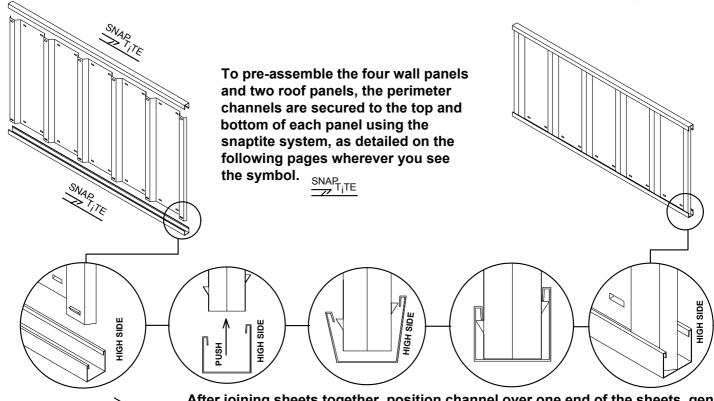
After joining sheets together, position channel over one end of the sheets, gently tapping it over the snaptite lugs, working along the sheets to the other end.
