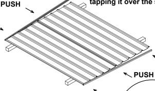
Each perimeter channel must finish flush with the edges of the sheets. The snaptite system allows adjustment for this process by simply tapping the channel along the sheets until each end is neatly flush. If you need to remove channels from the panels, pull the channel along the panel from opposing ends. You may need someone to help with this.
