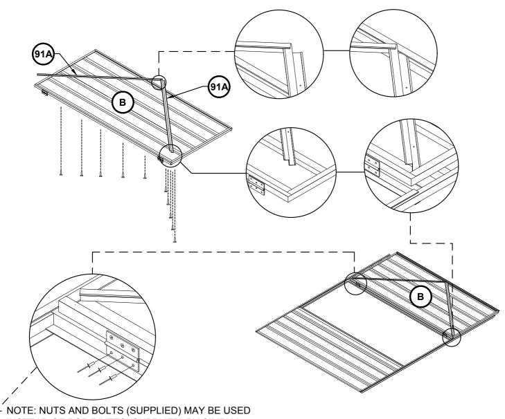
∠ NOTE: NUTS AND BOLTS (SUPPLIED) MAY BE USED INSTEAD OF POP RIVETS (SUPPLIED) BY SIMPLY ENLARGING THE HINGE HOLE SETS IN THE JAMB **USING A 4MM DRILL BIT**
