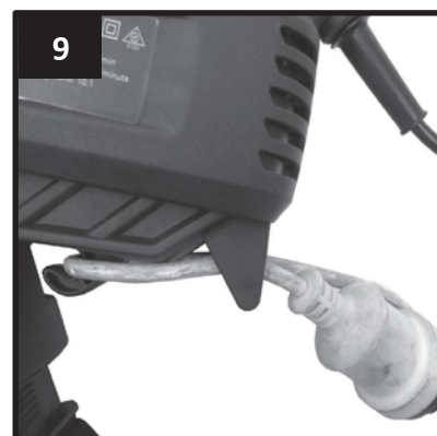
Make a loop with the extension cord and push it through the square hole under the motor housing and over cord retainer. Connect the extension cord socket to the blower vac's cord plug.
