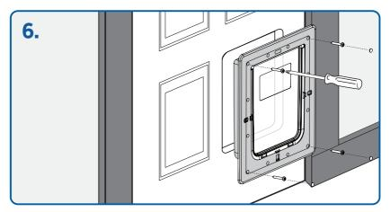
Place both frames into the opening and secure with screws and caps provided. Select the correct size screws below for your installation.
