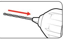
3 Tighten the chuck by turning clockwise.
