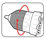
2 Insert the drill bit, making sure it is centred in the chuck.
