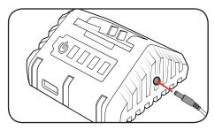
2 Slide the battery onto the cradle. The first 2 lights will illuminate when battery is properly connected and is charging.
