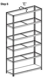
Apply remaining brackets as above to desired height. Ensure that braces 'E' are fixed to all shelves
