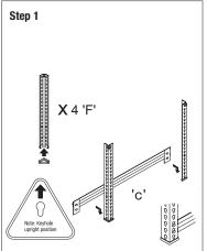
Place foot caps onto the bottom of the 4 legs 'F'. Note upright position. Place shelving bracket 'C' onto the legs 'F'. A rubber mallet can be used to lightly tap all brackets into the keyholes of the legs into place. Allow one keyhole free between the foot cap and the shelving bracket.
