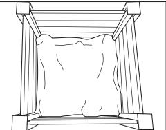
Lay the black geotextile fabric in evenly. Allow excess fabric to lay up the walls.
