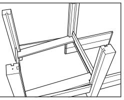
Place in notched boards and remaining base boards. The boards will sit at an angle
