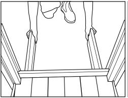
Once the base boards are installed, hold the 2 support boards and pull them out equally, this will lock the base in.
