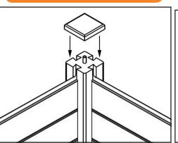
Insert the 4 hardwood dowels into the holes on the top of the posts by hand and then place 4 caps over these dowels. Push down to secure.
