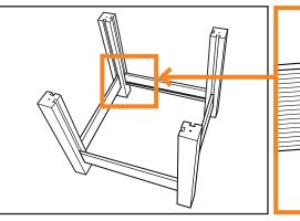
Ensuring the 8mm hole is on the top & the grooved (reeded) side of the timber boards is facing inwards slide in 2 standard & 2 slotted boards opposite to each other.
