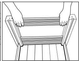
Slide in the remaining boards ensuring the branded board is on top. **Please note:** Hold the boards equally allowing the weight of the board to find the correct position.
