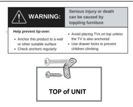
When attaching unit to wall put safety bracket in middle of unit with 16mm pan head screw then 25mm pan head screw into wall.
