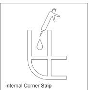
8. Peel back the protective film on the second panel just enough to allow it to slot into the plastic internal corner strip. Starting from the bottom, start fitting the panel into the plastic internal corner strip ensuring the panel is fully seated.
