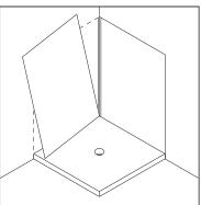
9. Once the adhesive is fully cured, remove the remaining protective film from the shower wall panels. Apply silicone sealant along the sides of the shower wall panels, as well as around the holes for the tap fittings.
