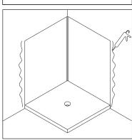
10. Apply silicone sealant to where the shower wall panel meets the shower base. Allow sealant to fully cure (refer to sealant instructions) before using the shower.
