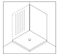
7. Run a bead of silicone along the length of the plastic internal corner strip for the second panel.
